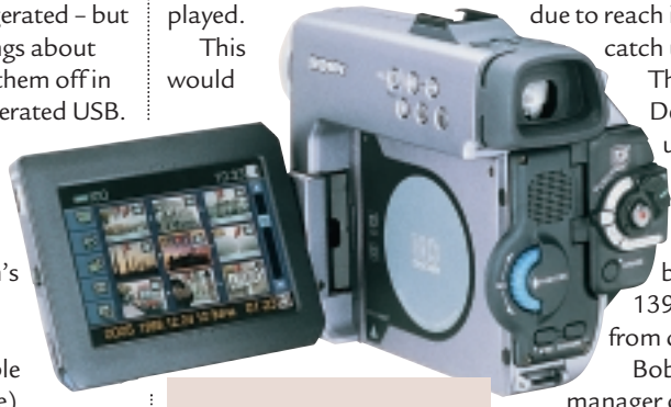
STRANGELY, SONY CHOSE NOT TO USE I.LINK IN ITS NEW DCM-M1 DIGITAL CAMCORDER. INSTEAD IT HAS AN OPTIONAL ETHERNET LINK
